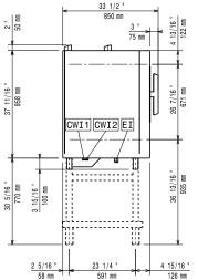
Cold Water inlet 1 (cleaning) CWII = Cold Water Inlet 2 (steam generator) CWI2
